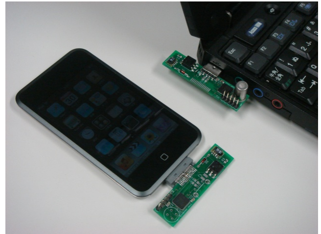
Figure 1. Appearance of “Parasitic Ambient Logger” System. (sensor modules attached to an iPod touch and a laptop computer)
