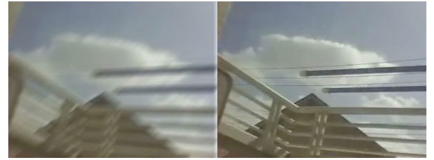
Figure 8: Video stabilization. (Left: raw image captured by mounted camera; right: image stabilized by video stabilization)
