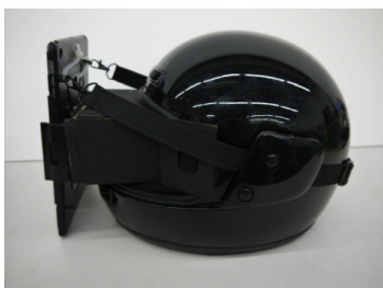
Figure 2: This is a prototype system of ChameleonMask. iPad air is held on full face helmet. Hacosco put in iPhone6 is set on eye part.
