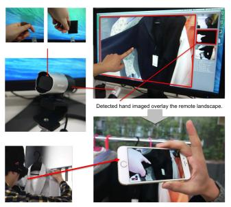
Figure 6. We use optical phenomenon on lcd display. A polarizing filter is attached on camera to detect hand from black background. Detected hand images are overlaid on the landscape the surrogate looks.
