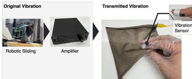
Figure 6: Experimental setup for the input–output vibration relationship (Evaluation 2). Finger vibrations were measured using the Picoleaf sensor (biodegradable piezoelectric sensor) [9] attached to the fingertip while participants rubbed the electrified cloth.
